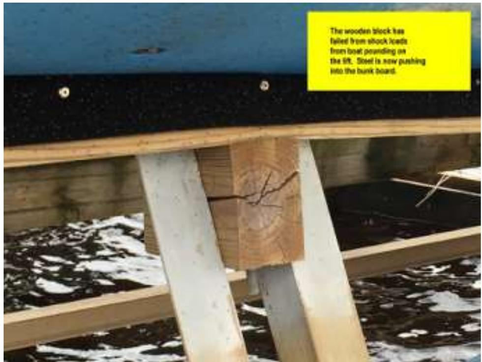
The wooden block has failed from shock loads from boat pounding on the lift. Steel is now pushing into the bunk board.
